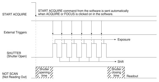
Figure 45. Multiple Trigger Timing Diagram
